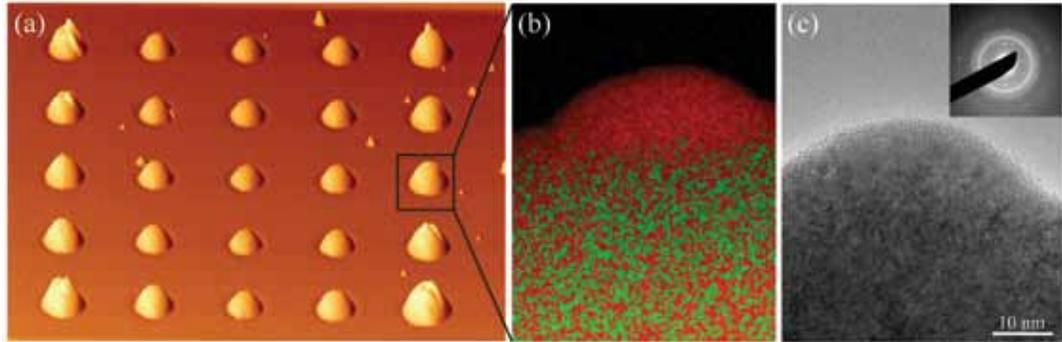
**Figs: (a) AFM image of 2-dimensional FIB-fabricated Ga droplet array on GaAs; (b) XEDS cross-sectional map of Ga (red) and As (green) in the vicinity of a Ga droplet shows that the composition of this droplet is pure Ga; (c) cross-sectional TEM image and corresponding diffraction pattern in the vicinity of a Ga droplet indicate that the structure of the Ga droplet is amorphous and there is a polycrystalline GaAs layer underneath the droplet.**
