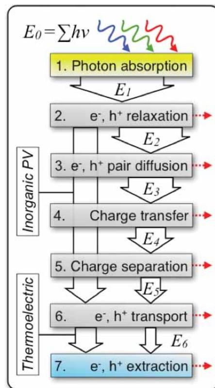
**An illustration of the multi-step, light-to-electricity conversion processes for organic PV, inorganic PV, and thermoelectrics. The loss mechanisms at each step are also described.**
