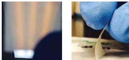
**Figure 1. Translucent and gently bendable thin films of lithium ion conducting ceramic electrolytes.**
