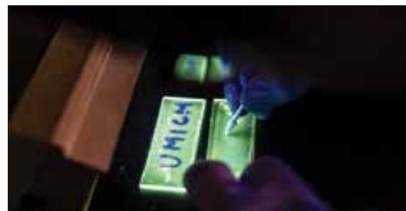
The purely organic phosphorescent thin film can reveal the presence of water under UV light. Water breaks hydrogen bonding between polymer matrix and embedded phosphors, changing from phosphorescent light (green) to fluorescent light (blue). Image credit: Joseph Xu
